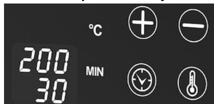
By default temperature 180°C is select. You can easily adjust the temperature as needed using the +/- buttons. Minimum temperature that can be selected is 50°C. Maximum temperature that can be selected is 200°C. Using the +/- buttons you can increase/decrease the temperature in 10°C increments. Your selection of the temperature as you adjust it will be displayed in the LED display.
